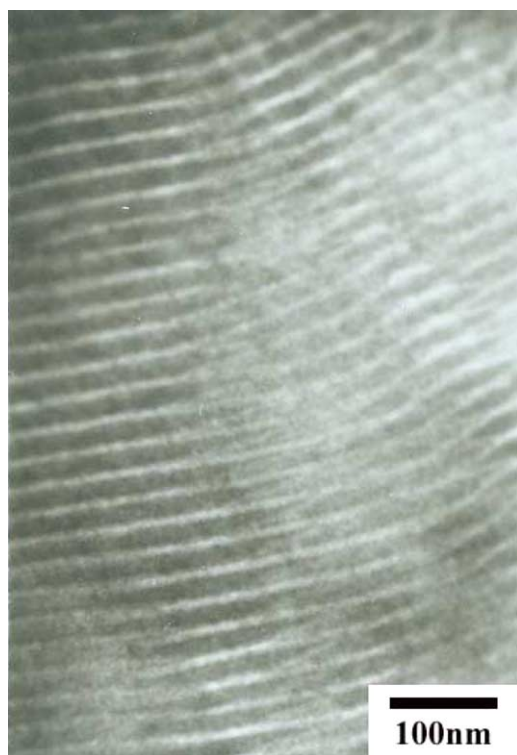
Fig. 11. The TEM image of a thin section of PCL 200 PMPCS 62 . The sample was sectioned followed by RuO 4 staining for 30 min. The dark regions are PMPCS and amorphous PCL domains, which were stained by RuO 4 .
